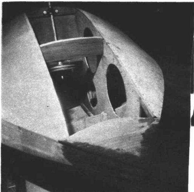
**TRIANGULAR** piece at front deck tip requires extra fairing. There's a tiller block that goes beneath it for additional support.
