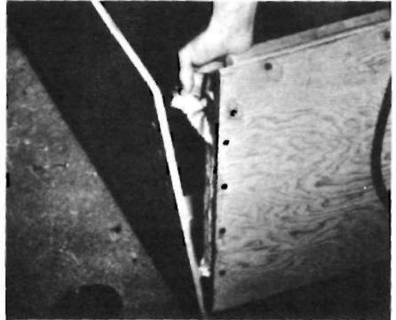
After drilling the sides for screws, glue them to the transom batten. Into the glue bed, lay linen strip which compresses, distributing the Weldwood marine glue entirely over the surfaces.
