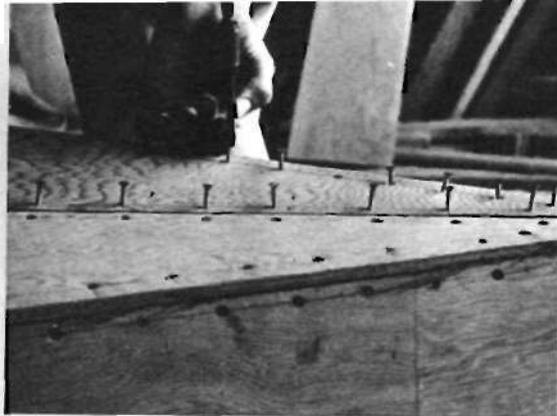
To strengthen hull, cover exposed bottom side joint with a strip of lumber for chaffing guard.
