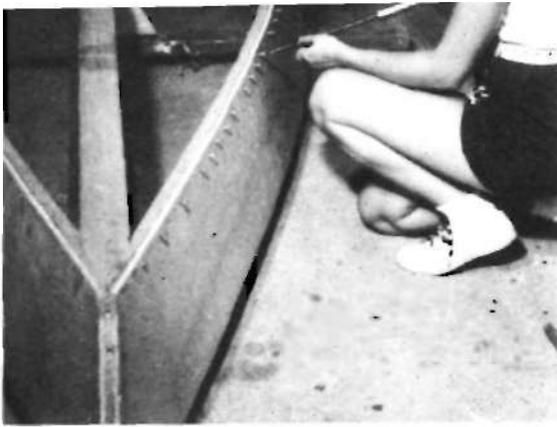
Ratchet screwdriver makes short work of setting the screws; no linen strips are used on the glued side joint since chine lace is milled at factory.
