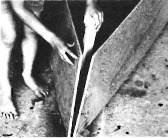
Inner stem Joins two sides at the bow, as shown here. This is planed to a bevel for a good fit, then glued and screwed in place. Get the stem absolutely vertical to avoid nose that is askew.
