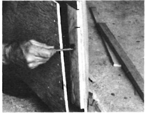
With the front bow aligned and drilled, glue and screw it closed, as described. Note that two chine rails with planed bevels are now ready to be wedged into place. Study the diagrams for details.
