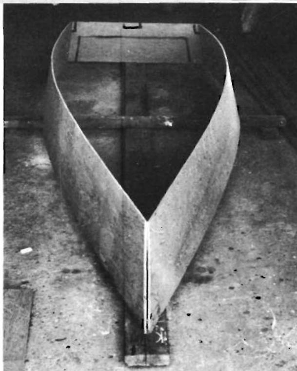
Photo at left shows the transom as seen on a jig, with the two side panels screwed lightly to it for bend trials; cord tacks front end, as shown here.
