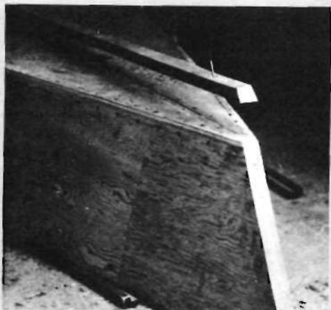
Outer keel goes on last, covers any gap between bottom halves, seals bottom, good launching skid.
