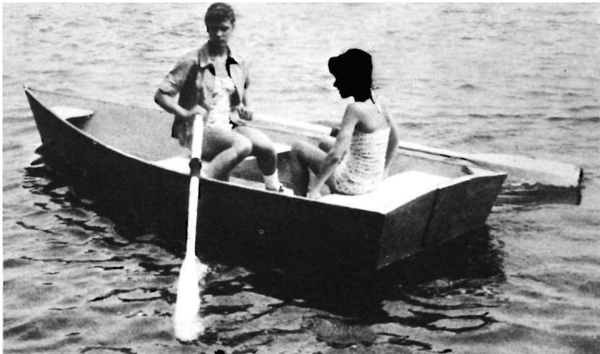
**T**HIS 11-foot hull will cost you only \$35 to build and comes out of a single sheet of  $\frac{1}{8}$ -inch plywood. We used Weldwood Royal Marine Plywood for the job. It can be put together by almost any workshopper with a minimum amount of tools and time.
