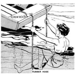
When using a rowboat as a diving platform, difficulty in getting into the boat from the water can be overcome by using the anchor chain as a step. The step can be made any height desired by using a screw hook to fasten it as indicated. A length of garden hose slipped over the chain will provide a cushion for the feet.
