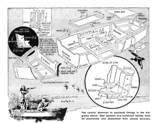
The seat rails are screwed to the frames in bow and stern sections, as shown above. The bow seat is screwed down, but the stern seat is hinged and forms a locker for fishing tackle, lunch, etc., out of the hot sun.
