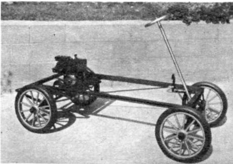
COMPLETED chassis and running gear with the brake pedal, brake rod, pedal-return spring, engine and drive assembly in place.
