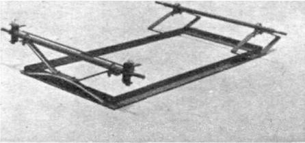
FRAME is cut from angle iron and welded together upside down. Front and rear axle and spring assemblies are bolted in place.
