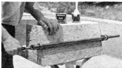
BODY for half-size 1901 Packard is made from half-inch plywood, glued and screwed at all joints and then clamped overnight.
