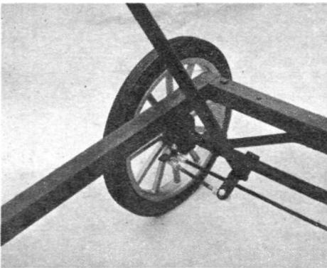
RIGHT front wheel detail shows steering assembly—shaft, pitman arm, perch welded to axle, drag link, tie rod and ball joints.
