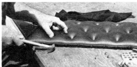
SEATS are plywood upholstered with one-inch foam-rubber covered with black Naugahyde and trimmed with half-inch edging.
