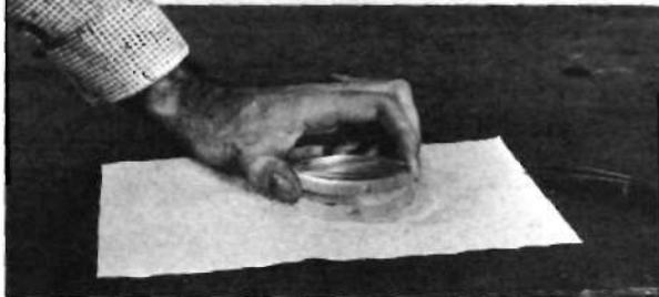
Separators provide air pocket between lenses. Place second lens carefully over one with separators. Both lenses should be resting on heavy tissue.
