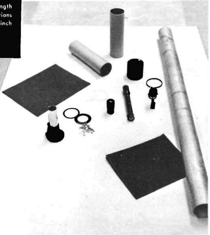
Lens-stops are of extreme importance in reflector, are cut from black paper after tracing size with compass.
