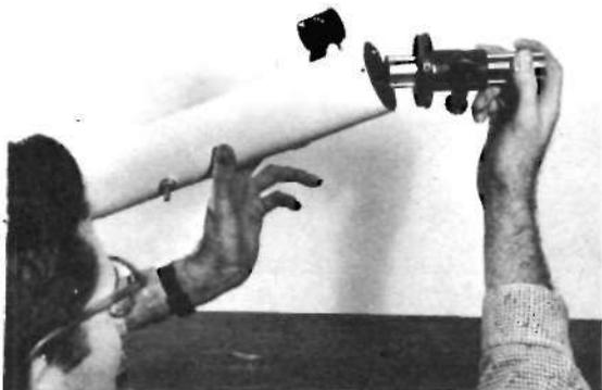
Rack-and-pinion eyepiece mounting comes next: it is inserted in rear end of tube, anchored in place by machine-screws through already drilled holes.
