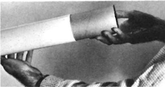
First lens-stop tube is slid into metal tube of telescope: cardboard tubes must be just the right diameter to fit snugly, can be bought for few cents.
