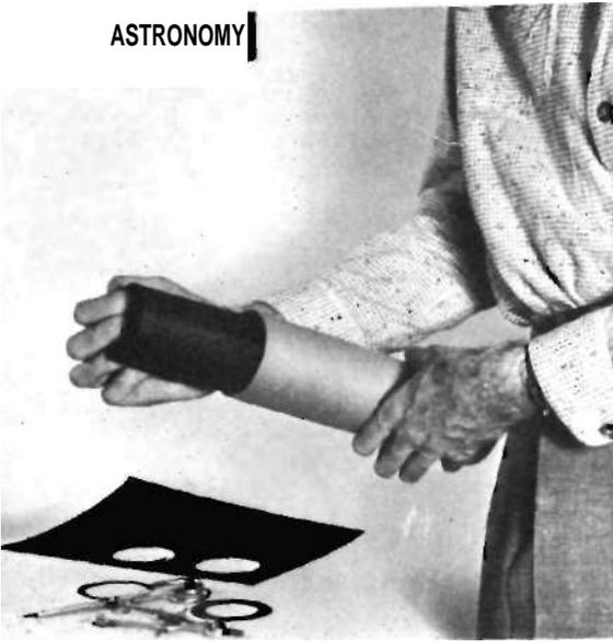
Lens-stops are cemented onto ends of cardboard tube, but first tube is deadened inside with black felt paper, which also is cemented and smoothed.
