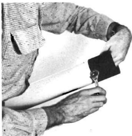
Long screws (1½ in.) should be used on previous steps, since screws will also serve to mount the telescope on tripod-head. But now attach lens-cell.
