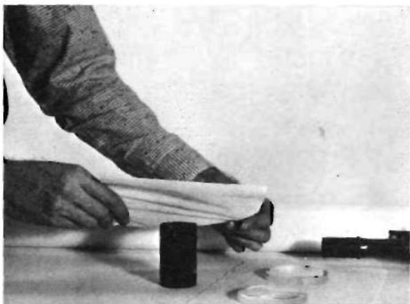
Another way to get lenses into cell is like this: using tin can or any sturdy cylinder as base, cover the cylinder with clean handkerchief, tissue.
