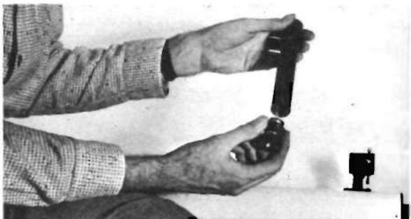
Eye-piece of small finder-scope is unscrewed so that finder-tube may be inserted through its mounting bracket, fastened to the aluminum telescope-tube.
