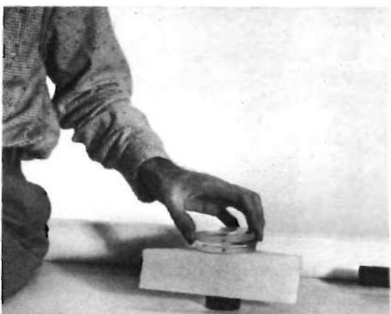
Place lens with separators in place on tissue or handkerchief. Then place other lens on top. Be sure that "flint" lens is on top. It is thickest.
