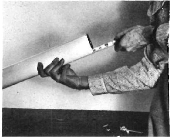
Measure distance to approximate center of inner stop-tube with long rule: hold scope-tube toward light, then peer inside and mark point on outside.
