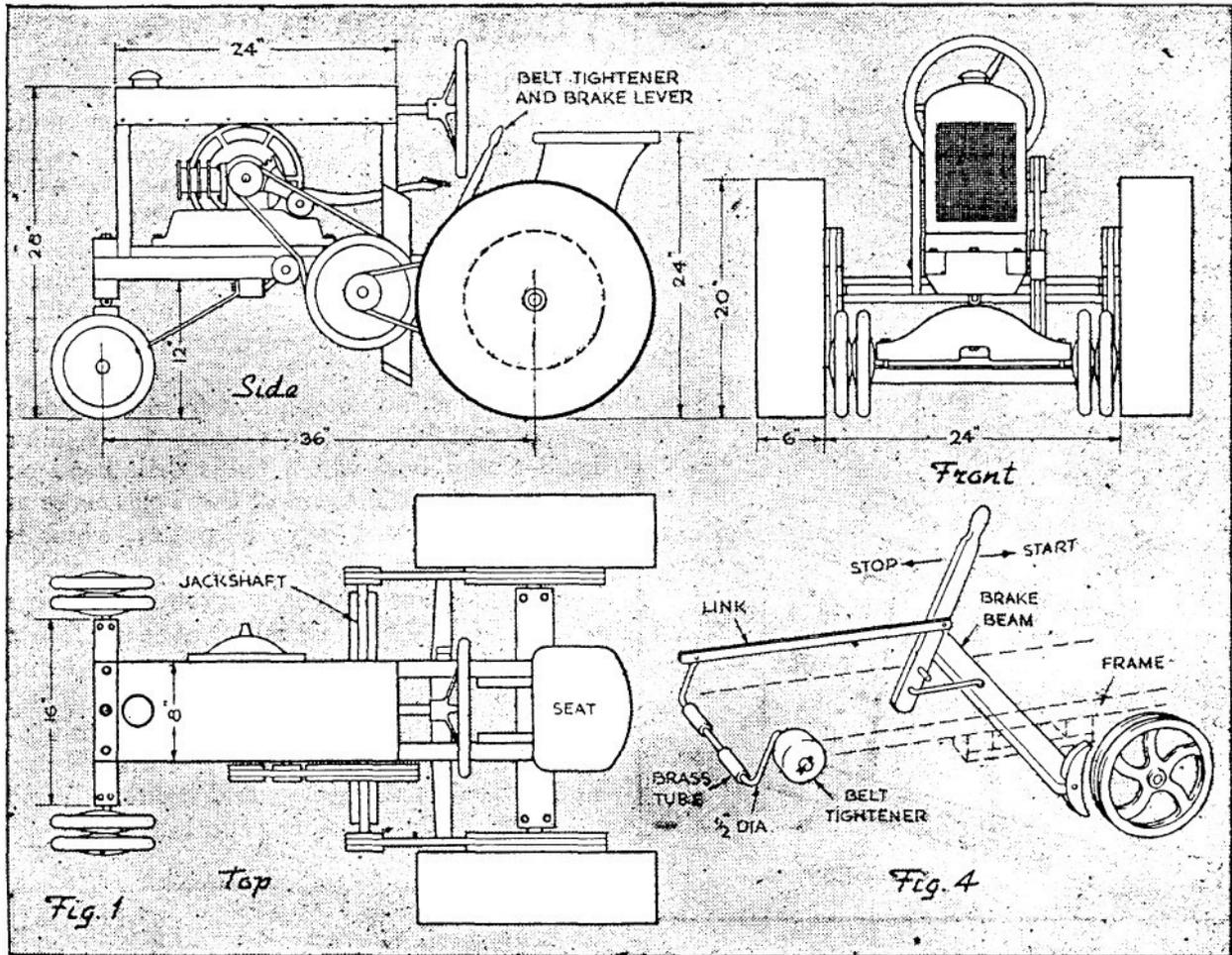
The rear axle is clamped to the two-by-three cross members by means of U-bolts, as is the front axle to its two-by-five inch member. The 3/4-in. steel jackshaft is carried in brass-tube bearings clamped to the frame with wood blocks as shown.
