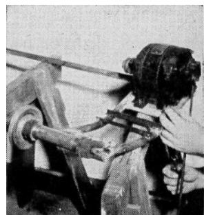
**Pouring yoke.** Cross members of the yoke are bent  $1\frac{1}{8}$ " below level of side members so that mixer-shatt bearings will be centered. Motor is  $1/3$  hp., 1,725 r.p.m., fitted with  $1\frac{1}{2}$ " pulley. Speed-reduction shaft and pulley ratio turn drum at 43 r.p.m.
