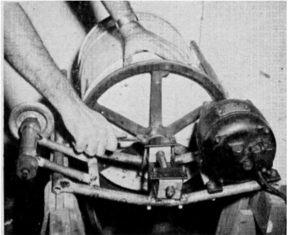
**Maple bearings**, soaked in oil and dusted with graphite, support drum shaft. Steel straps and J bolts secure bearings. With motor, drum and all parts in place, yoke is balanced to locate trunnions. These are welded 4" forward of balance point so drum swings up.
