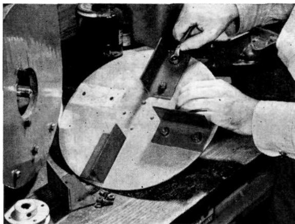
**4 Rotor blades,  $3\frac{1}{2}$ "** matched lengths of  $\frac{1}{8}$ " by  $\frac{1}{2}$ " by  $\frac{1}{2}$ " angle iron, are mounted with  $\frac{1}{4}$ "-20 bolts. Blades are spaced  $90^\circ$  apart with vertical flanges radial to center of disk and the ends all equidistant from disk edge. Hub must be carefully centered for good balance.
