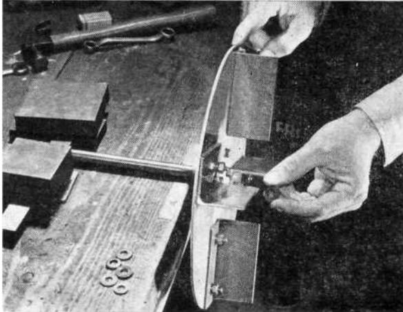
**5 Balancing the rotor.** Rest a 5/8" shaft on steel rule at edge of bench; weight down second rule over end of shaft. Slip washers on bolts until rotor stops at different place every time you spin it. Then take off nuts and clamp washers on.
