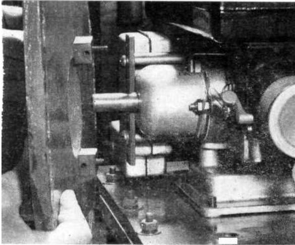
**2 Back plate of rotor housing**, cut to shape shown in drawing, was then fastened to strap iron. Two 1/4"-20 screws, run through plate and wood spacing blocks, were turned into holes tapped in strap ends. Plate was also bolted to angle iron bolted under base.
