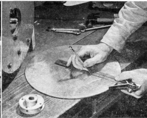
**3 Rotor** consists of 12 1/2" disk cut from 1/8" aluminum, a 3" cast-iron V pulley (used as a hub) and four heavy angle-iron blades. Here, disk center is being found with combination square. I avoided a die-cast pulley for hub; it might fly apart under centrifugal force.
