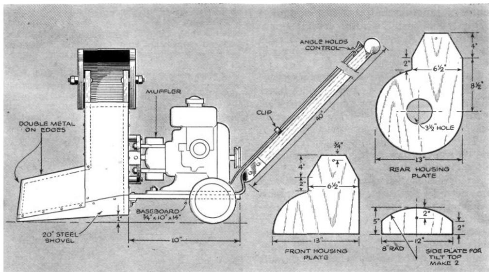
—a 1.2-hp., two-cycle job—from mower to plow.
