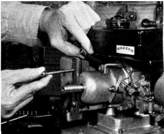
**1 Engine was mounted** with shaft projecting beyond one side of  $\frac{3}{4}$ " by 10" by 14" baseboard, bolts holding it in place. To support rotor housing, a piece of strap iron was attached to governor-shell boltholes. Two long screws and pipe spacers hold it alongside shaft.
