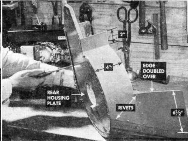
**6 Making the scoop.** Rear housing plate was removed to attach scoop and housing sides. Steel snow shovel was bent at rear to conform to housing curve. Tabs cut in edge were bent over and fastened to plate with wood screws. Wings were riveted to scoop sides, housing rim.
