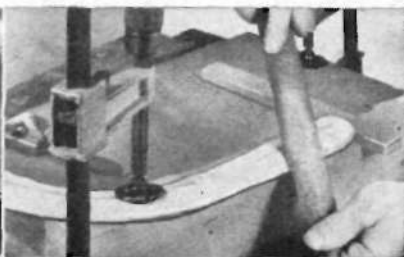
Round the top surface with a wood rasp and sand smooth
