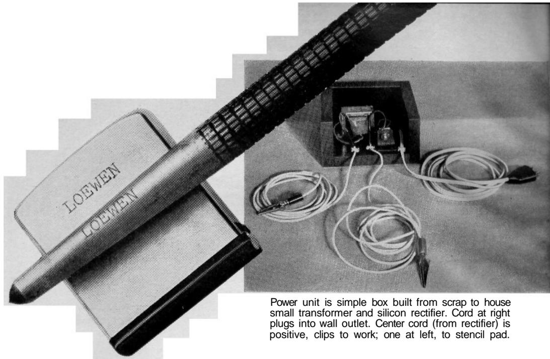
Power unit is simple box built from scrap to house small transformer and silicon rectifier. Cord at right plugs into wall outlet. Center cord (from rectifier) is positive, clips to work; one at left, to stencil pad.
