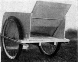
the front panel in place and serve as guides for sliding it up for dumping. Sides are notched to fit over the cross members of the frame. Eye hooks on each corner lock into screw eyes on the frame to hold the body in place.—W. M. Bosch, Rumson, N. J.
