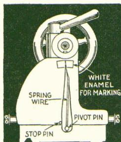
It consists of a sheet-metal pointer pivoted to a pin in the lathe bed, and a length of spring wire, which is fastened rigidly in the pin and wrapped around the pointer. The
