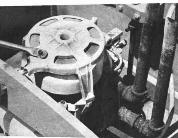
COOLING WATER exits through hose curling around exhaust pipe and passing through hole near top of transom.
