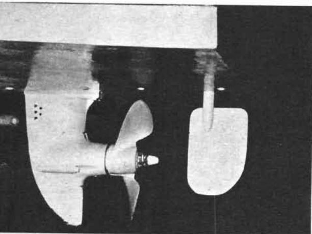
drove it along at 30 mph. However, it was later decided that a cut-down 5-hp Scott-Atwater outboard would be ample, giving a speed of 25 mph. Since the load is light, this engine will turn up to its peak of 4200 rpm, but it is wise to adjust the throttle so that continuous operating revolutions will be somewhat less.
