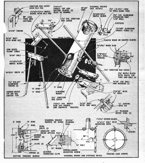
A RICH-FIELD telescope is an instrument that covers a fairly large segment of the sky and has good light-gathering ability. For viewing nebulae, the Milky Way and the moon, it can't be surpassed. The best RFT (richest-field telescope) of the reflecting type is one having a 7-inch diameter mirror of f-4
