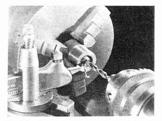
Stock for the crosshead is turned to a sliding fit in the main-column bore; then one end is recessed and turned to shape. The piece is also drilled and tapped for the piston rod while chucked.
