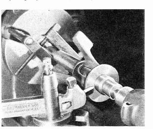
The column is then mounted on a mandrel held between centers for facing the head square with the bore and turning to diameter. It is next reversed on the mandrel and the feet faced smooth and true.
