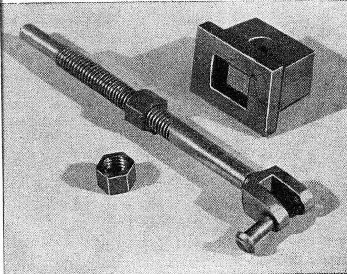
The slide valve is located on the valve rod by a pair of locking nuts that provide travel adjustment. The nuts must be a tight fit on the thread.
