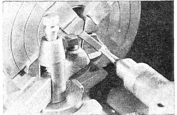
Chucked in the four-jaw, a piece of 1/4" square steel is turned down to form the handle of the reverse lever. Holes must be located as in the drawing.
