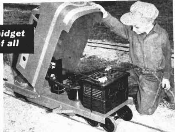
ELECTRIC-POWERED "DIESEL" made for use on strap-iron rail comes ready to roll. It has two forward and two reverse speeds. A trickle charger is provided to boost the 6-volt auto battery from the house circuit overnight. Both this and the gas-powered locomotive below are equipped with an electric horn and headlight.
