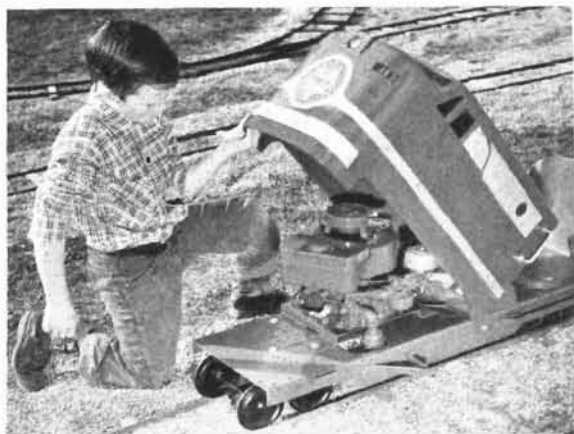
A FOUR-CYCLE TWIN powers this gas-driven locomotive. The throttle is spring-tensioned to snap shut when not held, providing a "dead-man" control for safety. Priced at $225 each, both engines above have bodies made of pressed steel and fiber-glass, finished in red and silver.
